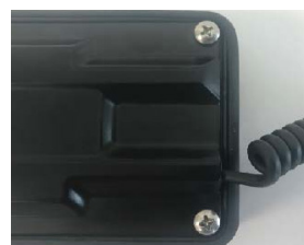
Sensor cable fed through the slot
